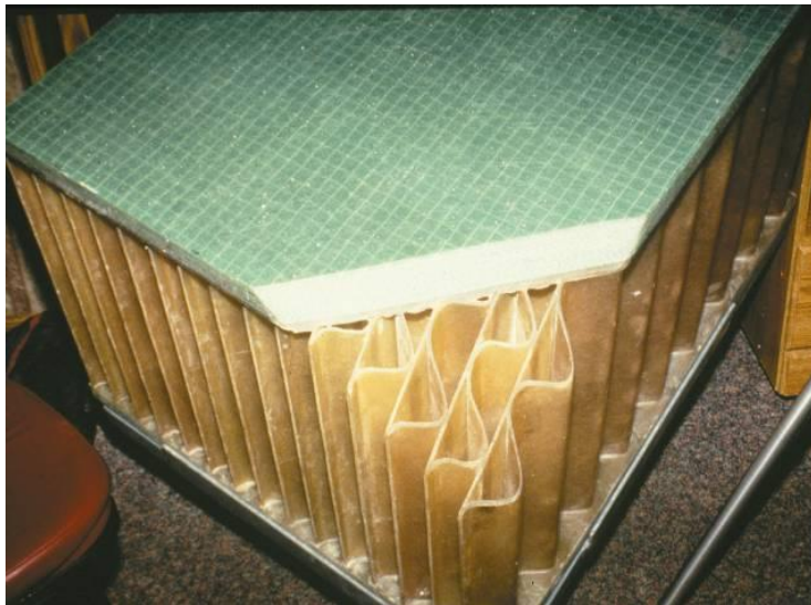
Structure of the Kansas panel
